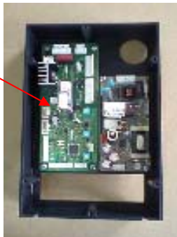
Main Control P.C.Board
