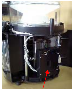
Control PC Box
